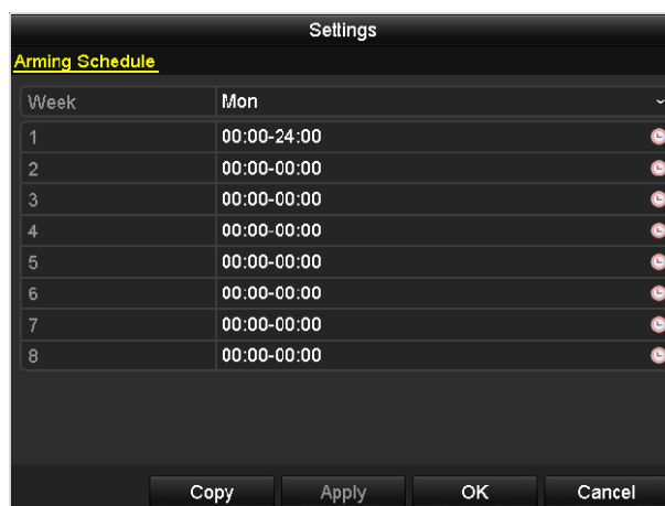
Figure 8-20 Set Arming Schedule of Alarm Output
